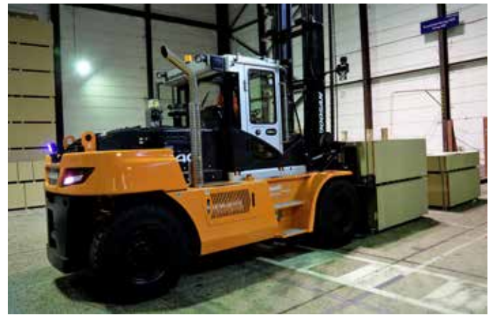
The new 14 tonners are equipped with a full cabin and lighting, a central lubrication system and comply with Euro Stage IV emission standards.
