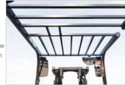
The neatly arranged hydraulic hoses and chains provide clear front visibility through the wide view mast.
