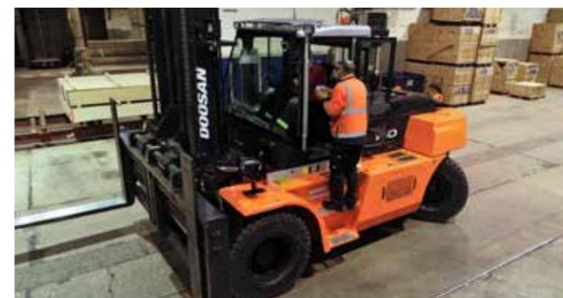
Thanks to the large anti-slip step plates, the Zeus cabin is safe and easy to mount and dismount. For educational purposes, the cabin is equipped with an extra seat for instructor.
