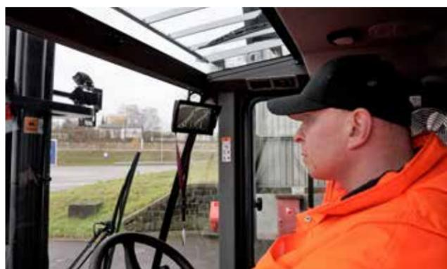
The Zeus Cabine has slim A- and B-pillars for optimal all-round visibility. Meanwhile, the front and rear view cameras also keep an eye on things.
