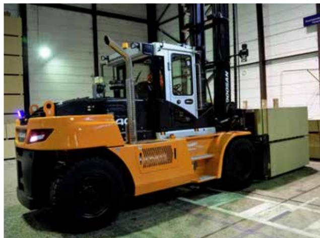
The new 14 tonners are equipped with a full cabin and lighting, a central lubrication system and comply with Euro Stage IV emission standards.
