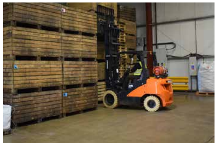
The G35C-7 has a 3-stage free-lift mast well suited for stacking heavy boxes of onions up to 6m high.
