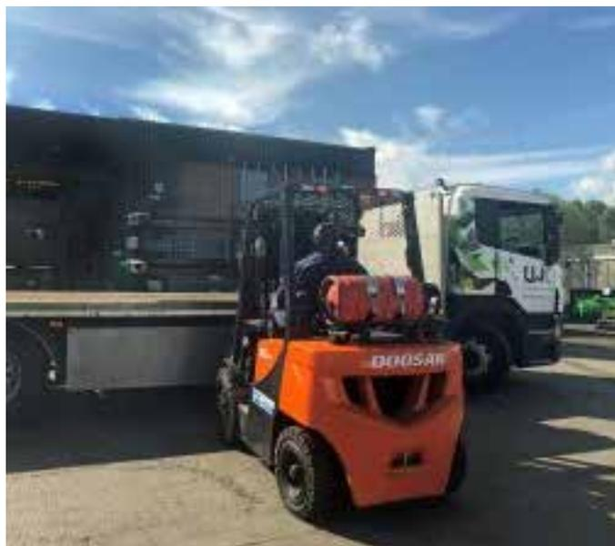
a Doosan G35C-7 3.5 tonne forklift. All were gas powered for continuous shift indoor operations.
